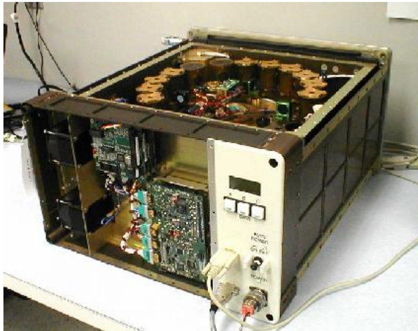
Figure 1. Picture of SHOT's Avian Development Facility (ADF) showing 18 positions for holding samples. There is an identical carousel below (see Figure 2). The two carousels rotate independently and are served by a chemical robot that injects reagent solutions into one sample at a time on a predetermined program or by remote control. Each sample holder also rotates independently of carousel rotation.
