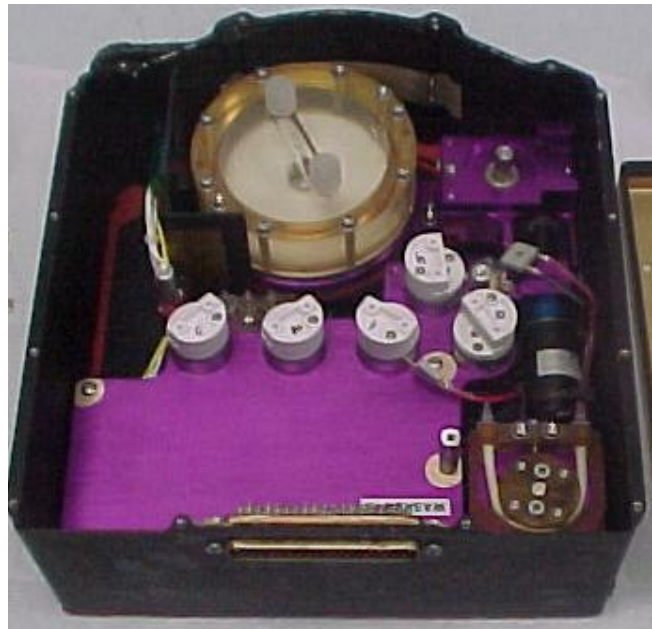
Figure 6. Photograph of CELLCULT bioreactor system integrated into SHOT's standard ADSEP cassette envelope. The gasket around the outer edge provides one of the two or three levels of safety containment.
