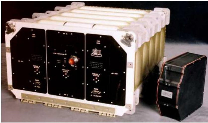
Figure 3. Photograph of a closed cassette and of the ADSEP biotechnology facility.
