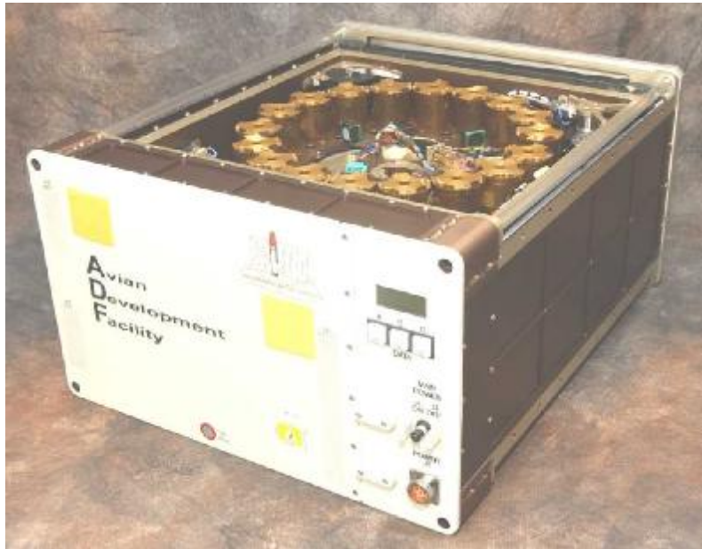
Figure 7. Picture of SHOT's Avian Development Facility (ADF) showing 18 positions for holding samples. There is an identical carousel below. The two carousels rotate independently and are served by a chemical robot that injects reagent solutions into one sample at a time on a predetermined program or by remote control. Each sample holder also rotates independently of carousel rotation.
