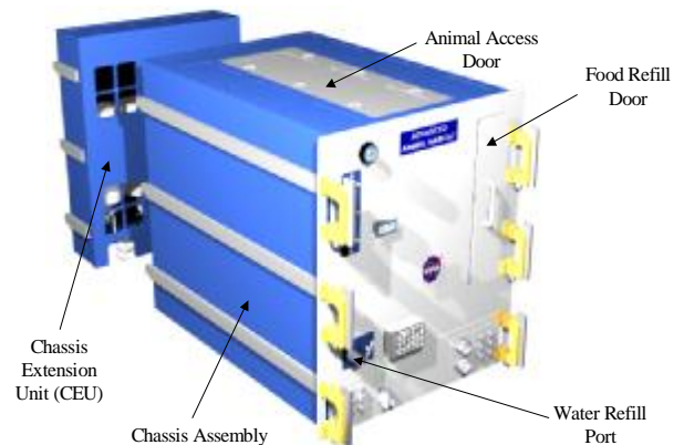
Figure 1. Exterior design of the AAH – C. The main chassis is compatible with all space vehicles. For use on ISS the Chassis Extension Unit (CEU) is attached at the rear of the chassis and is used to store supplies and to effect heat transfer to avionics air.
